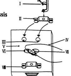
Note: The safety rope must be able to withstand 12 times the weight of the lamp, and the extension cannot exceed 20cm.
